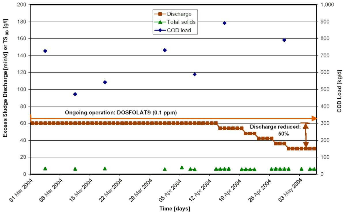
**Figure 5: The MEG sewage treatment plant - COD load as activation load magnitude, reduction of the excess sludge discharge as well as the equilibrium solids content in the activation tank**
