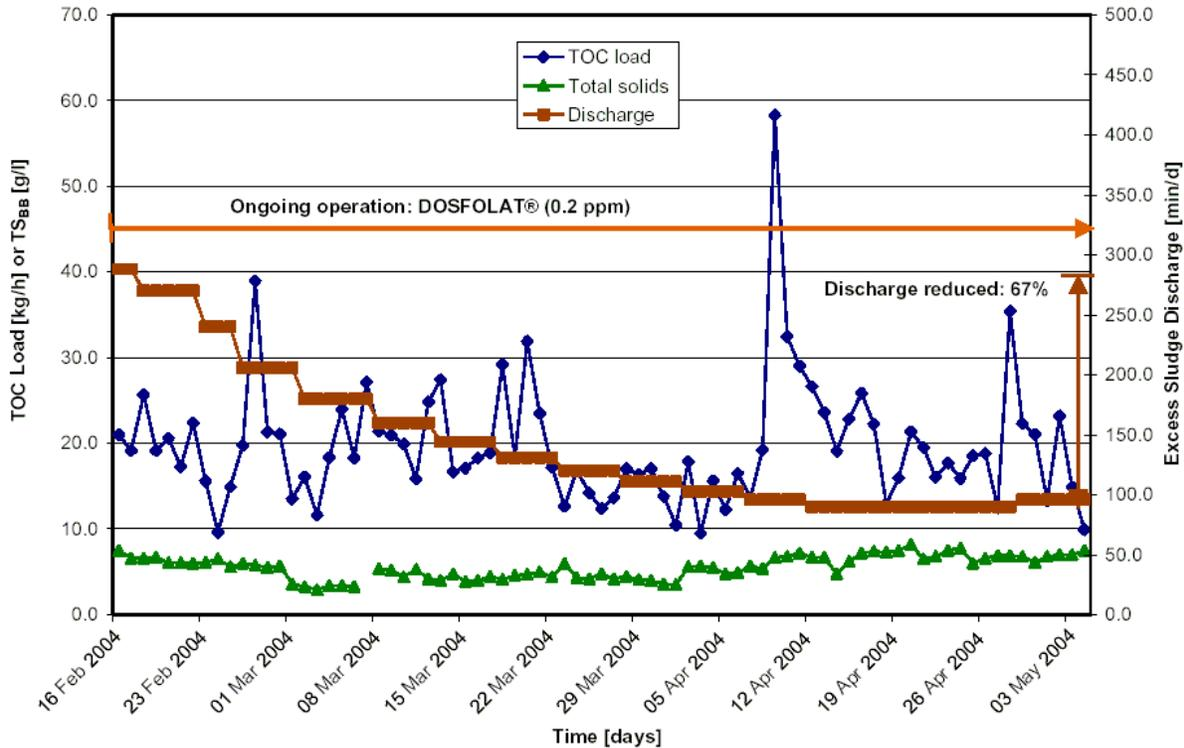
**Figure 4: ISP sewage treatment plant - TOC load as activation load magnitude, reduction of the excess sludge discharge as well as the equilibrium solids content in the activation tank**
