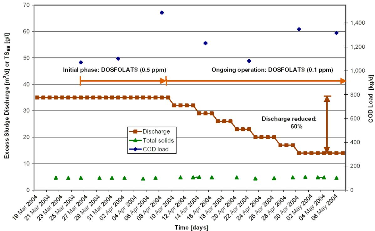
**Figure 6: The treatment plant LSP - COD load as activation load magnitude, reduction of the excess sludge discharge as well as the equilibrium solids content in the activation tank**
